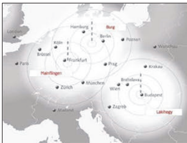
Figure 1 - Ripple control transmitters
